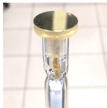
Figure 2.1-1. Single-crystal Au(111) electrode in a glass capillary.
