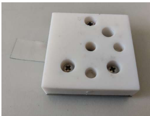
Figure 7-4. Photo of the electrochemical cell.
