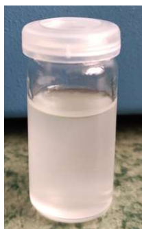
Figure 9-9. Emulsion consisting of 100 \mu l of 5 mM DMFc and 400 mM P (6,6,6,14) N(Tf) 2 solution in toluene and 5 ml of 0.1 M HClO 4 aqueous solution after preparation [278].
