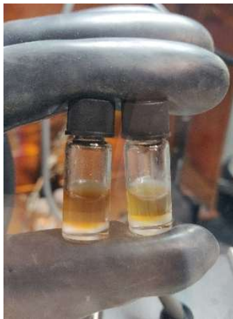
Figure 7-32. The picture of biphasic system consisting of 5 mM LiTB in 0.1 M HClO 4 aq. and 5 mM DMRC 5 mM BATB in NPOE, with stirring 500 rpm, picture was taken after the weekend of employing UV light (left flask), after the weekend without light (right flask), in glove box.
