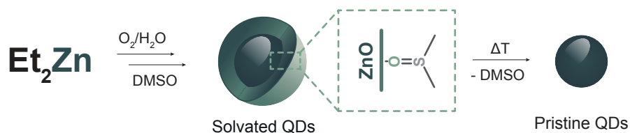
Figure 1.16: Schematic representation of the one-pot-one-step organometallic synthesis of DMSO-QDs.
