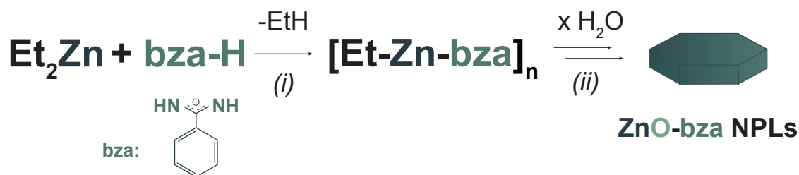
Figure 1.23: Schematic representation of one-pot self-supporting organometallic (OSSOM) procedure for the preparation of ZnO NPLs.
