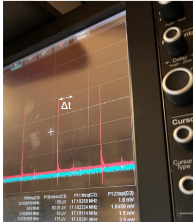
Figure B.1: Synchronization between the cavities using the oscilloscope.
