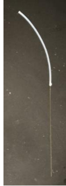
Figure A1.5: Shows the final device with the glass capillary inserted and fixed. On the right, the glass capillary (inner diameter: 40 \mu\text{m} ) is glued to the tubing.
