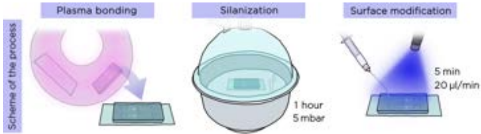
Figure 4.1: Scheme of hydrophilic surface modification: following standard plasma bonding of the chip, we depose vapours of Silane on the surface, positioning the chip in a vacuum chamber with 30 \mu\text{l} of Vinyltrichlorosilane for 1 hour. Finally, we flush the GelMA solution inside the channels while using UV light to promote the bonding between GelMA polymers and the Vinyltrichlorosilane.
