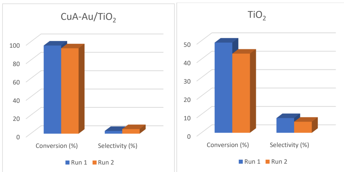
Figure S11. Photocatalytic experiment with CuA-Au/TiO 2 ( left ) and sol-gel synthesized TiO 2 ( right ) (Run 1) and after washing the catalyst with ACN and H 2 O (Run2) under UV irradiation (60min) in batch system with ConOH .
