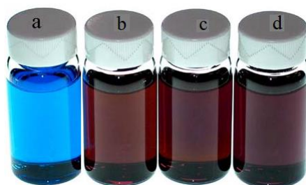
Figure 4. Effect of phthalate isomers on color changes of 2 : (a) 2 ; (b) 2 +phthalate; (c) 2 +isophthalate; (d) 2 +terephthalate. Adapted with permission from the Elsevier. Copyright 2006. 5
