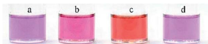
Figure 65. Effect of maleate and fumarate anions on color changes of 60 : (a) 60 ; (b) 60 with 0.1 equiv. of maleate; (c) 60 with 2.0 equiv. of maleate; (d) 60 with 2.0 equiv. of fumarate.
