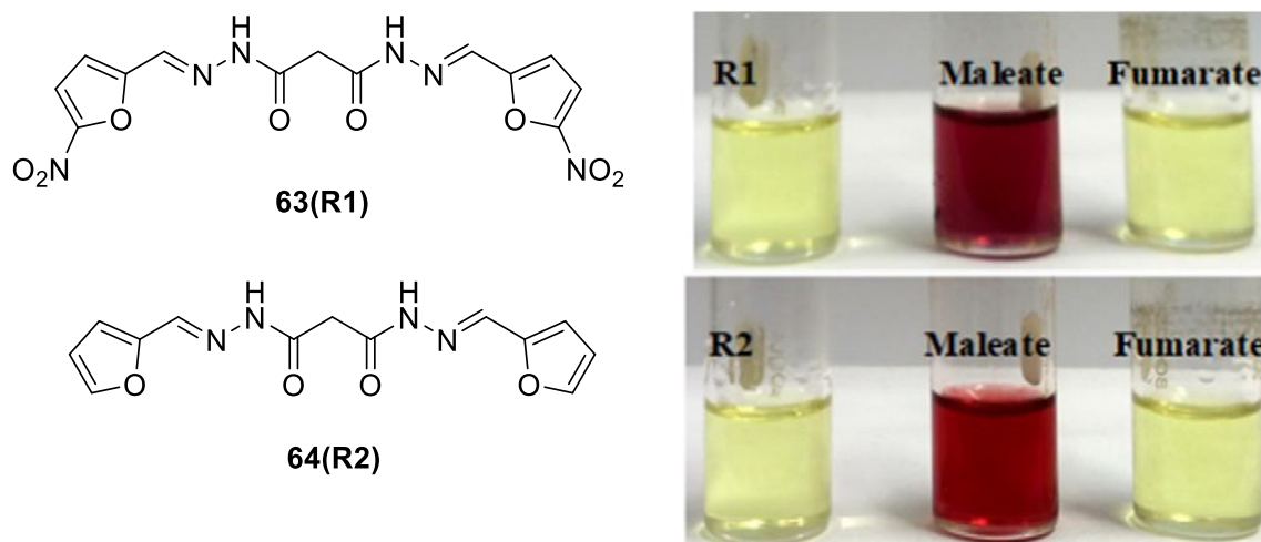
Figure 68. The molecular structures of receptors 63(R1) , 64(R2) and their solutions in the presence of maleate and fumarate. Adapted with permission from the Elsevier. Copyright 2020. 108
