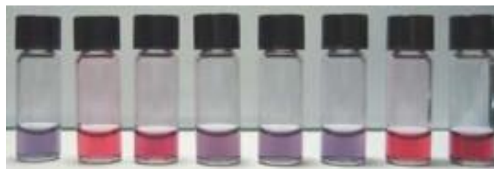
Figure 31. Color change of AuNPs 26 upon addition of analyte. From left to right: fumarate, maleate, oxalate (C2), malonate (C3), succinate (C4), glutarate (C5), propionate and 4-pentenoate. Adapted with permission from the Elsevier. Copyright 2008. 72
